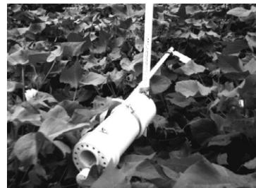
Figure 1. Micro-station inside the cotton crop with the air temperature, relative humidity, and LWD sensors.
