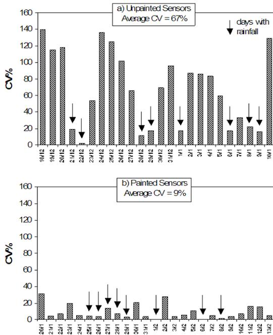
Figure 2. Coefficient of variation (CV%) for the LWD measurements using electronic leaf wetness sensors unpainted (a) and painted (b). The arrows indicate the days with rainfall.
