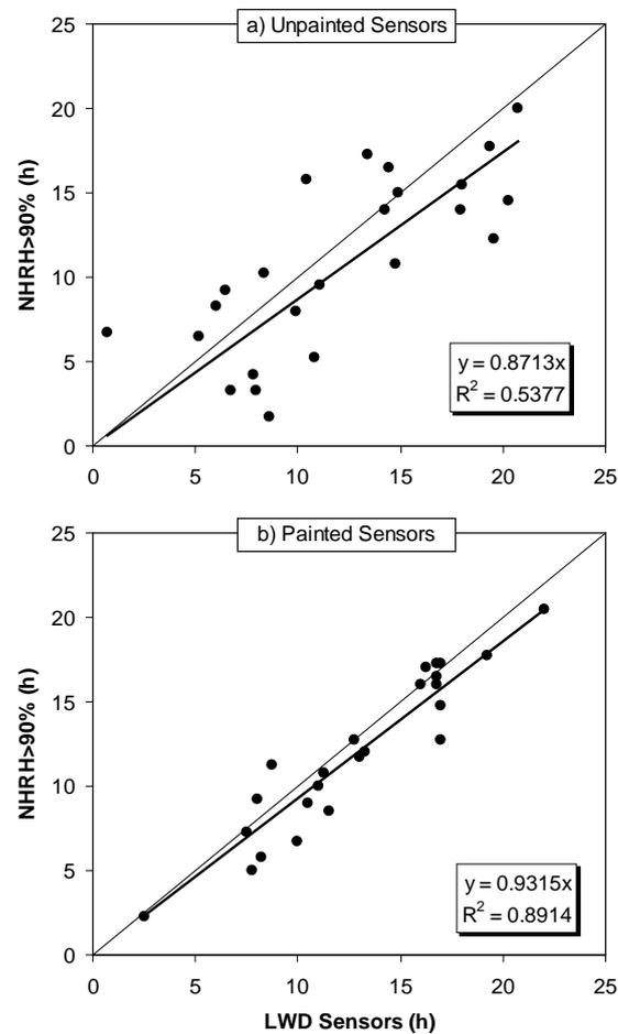
Figure 3. Relationship between the measured LWD (mean for the six sensors) and NHRH>90% with the sensors unpainted (a) and painted(b).
