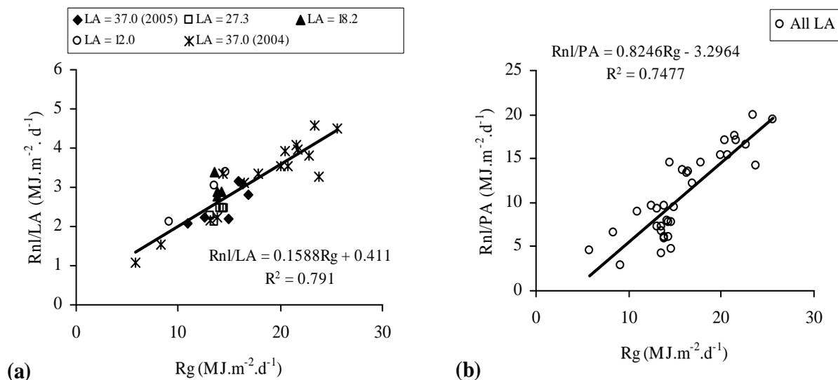
**Figure 6.** Relations between daily values of orange canopy net radiation by leaf area unit (Rnl/LA) and global solar radiation (Rg), with data points being showed separately for each leaf area and the two years (a), and with pooled data between tree net radiation per area unit canopy projected on the soil (Rnl/PA) and global solar radiation (Rg) (b).
