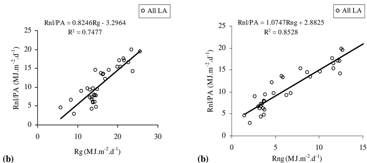
**Figure 7.** Relations between daily values of orange canopy net radiation per leaf area (Rnl/LA) and grass net radiation (Rng) for all leaf areas (LA) (a), and between orange canopy net radiation by area unit projected by the canopy on the ground (Rnl/AP) and grass net radiation (Rng) for all leaf areas (b).
