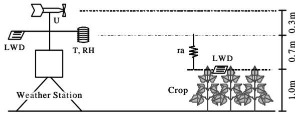
**Figure 2.** Schematic of the sensor's height and the additional resistance required by the RES model.
