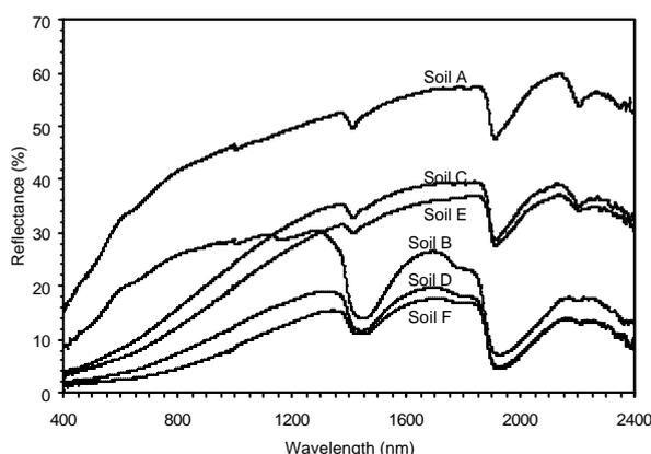
**Figure 2.** The spectral signature of the soils.
