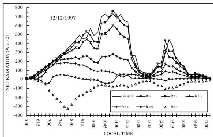
**Figure 2.** Time course of the non-weighted net radiation flux density for six sensors around the citrus tree with the equilatitudinal setup, and above grass net radiation.
