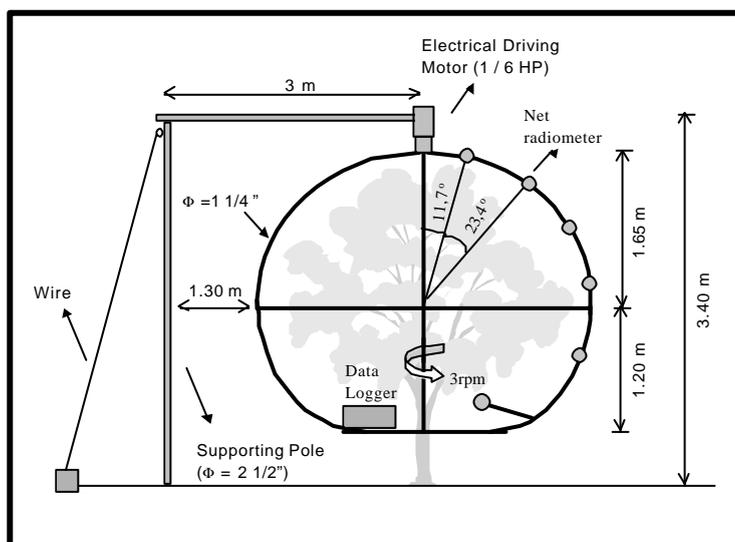
**Figure 1.** Scheme of the device used for the citrus tree net radiation measurements (Setup 2).
