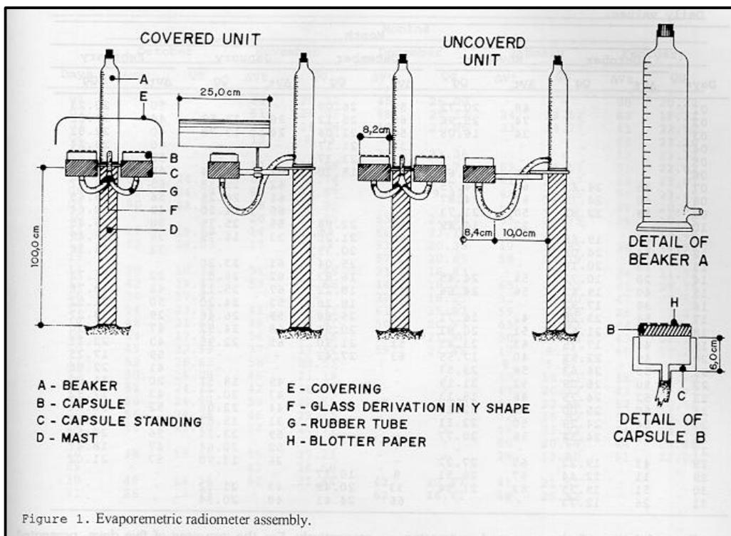
The clay capsule (B) did not suffer action of capillarity effect. There was a small hole in its middle whose main function was to expel the air out from the tank and allow the checking of the water level. The capsule standing (C) and the mast (D) were made by conduit tube and painted dim white.
